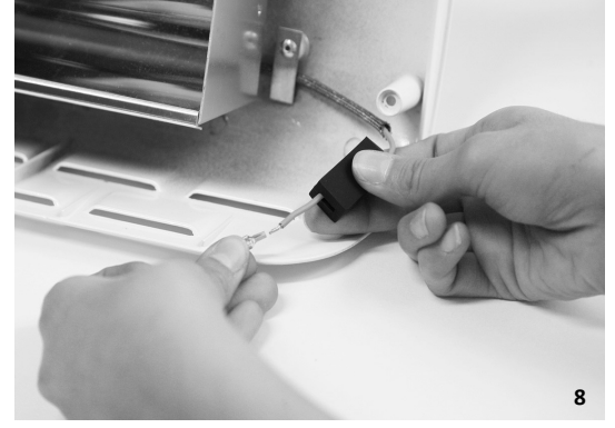
8. APPLY THE NEW SPARE FASTONS AND FASTEN THEM TO THE CORD.
