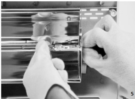
5. REMOVE THE 2 BULB EXTREMITY HEAT-ELASTIC CAPS AND DISCONNECT THE TWO FASTONS CONNECTING THE CORDS TO THE BULB (IF THE CAPS USED DISPLAY SIGNS OF WEAR AND TEAR, THESE MUST BE REMOVED BY CUTTING THE CORDS NEXT TO THE TWO FASTONS).
