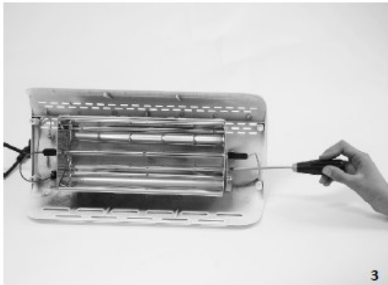
3. UNSCREW THE SCREWS HOLDING THE TWO SMALL SIDE PROTECTION COMPONENTS.
