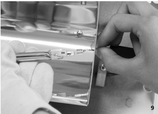
9. CONNECT THE MALE FASTONS OF THE NEW BULB TO THOSE OF THE TWO CORDS. COVER THEM WITH THE CAPS AND RE-POSITION THE BULB IN THE SEAT OF THE TWO SPRING CLIPS. DO NOT TOUCH THE BULB WITH YOUR BARE HANDS.
